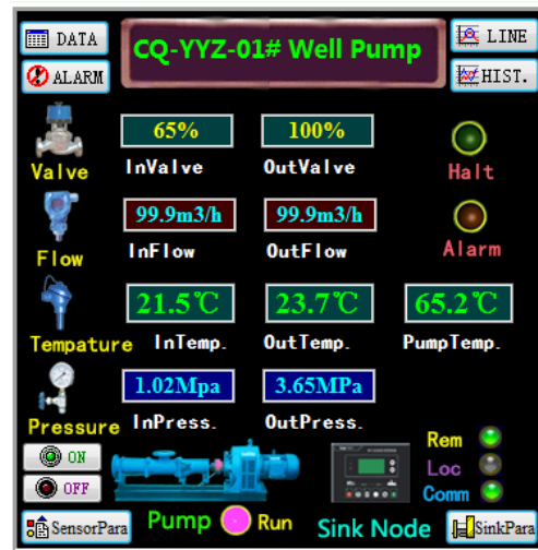
Figure 6. Remote monitoring main screen of the petroleum well based on IOT technology
