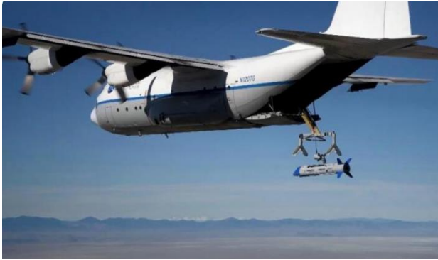
Figure 5. A C-130 transport aircraft carrying a Gremming drone
