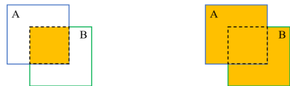
Figure 6. Schematic diagram of intersection and concatenation of IoU prediction and real frames.
