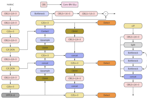
Figure 4. YOLOv8s+DCN+CBAM Network Architecture
