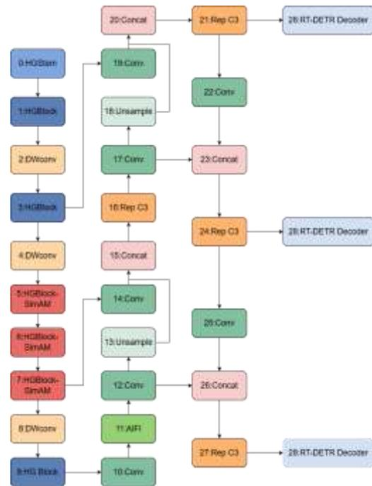
Figure 2. Network architecture of improved RT-DETR
