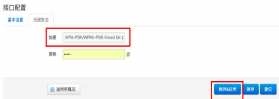
Figure 17. Encryption configuration
