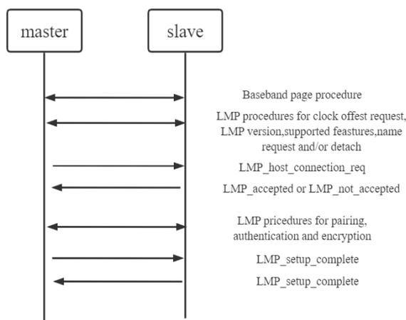
Figure 1. Bluetooth pairing process diagram
