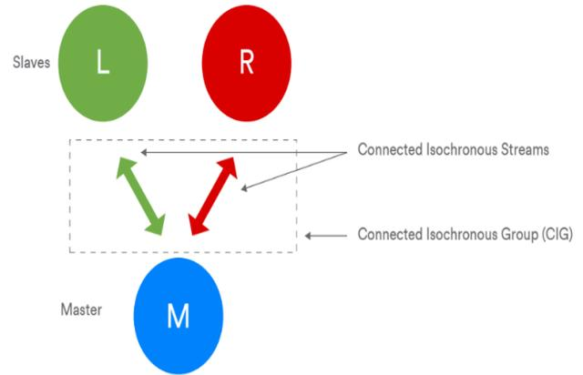
Figure 5. Isochronous channel diagram in connection mode
