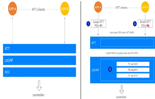
Figure 4. The relationship between ATT and L2CAP is about MTU
