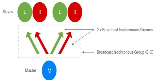
Figure 6. Isochronous channel diagram in broadcast mode
