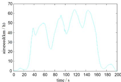
Figure 4. Soft threshold method airspeed denoising curve diagram.
