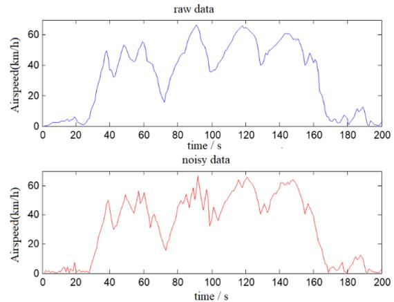
Figure 3. Airspeed raw data, noise data curve change diagram.
