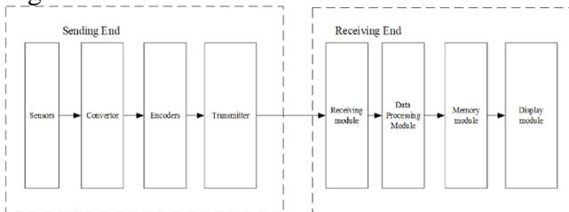
Figure 1. Overview of telemetry data processing structure.
